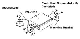
• Make sure to use the supplied flush head screw  $(M4 \times 3)$  to install the monitor.
